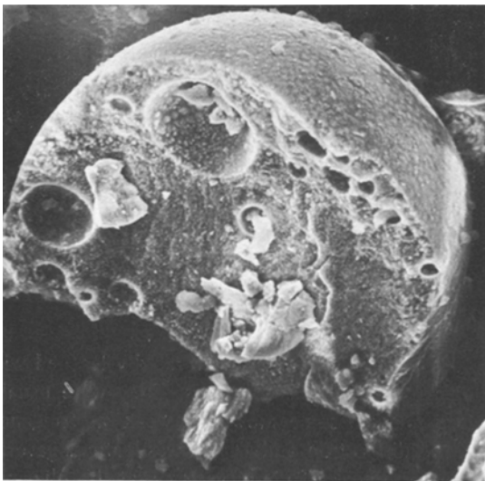
Figure 13 A broken type III spheroid showing its highly porous nature. SEM, \times 950 .
